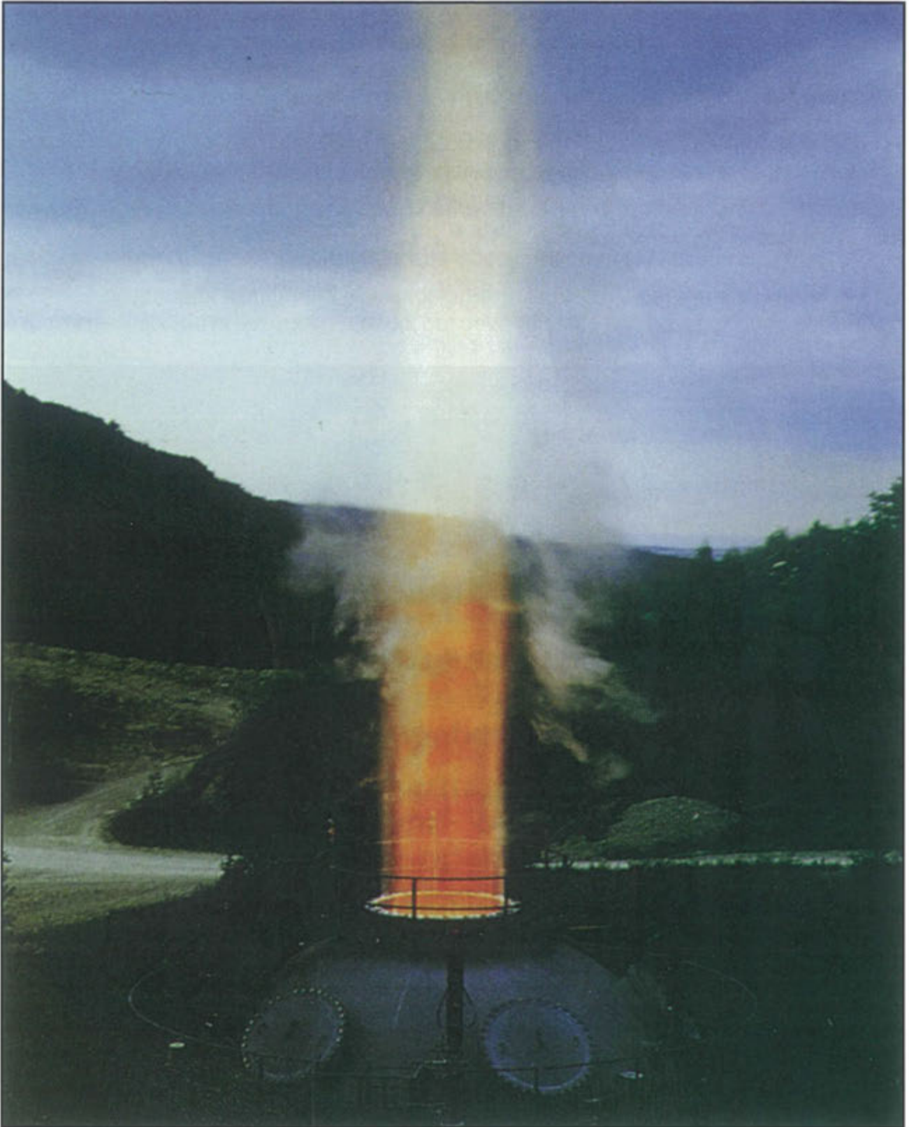
Fig. 16: Explosion venting of a 250 m 3 vessel Rapidly developing dust explosion ( K_{St} -value = 300 bar · m · s -1 ) in a vessel with a small venting area results in a high, reduced explosion overpressure whereas the pressure generated outside the vessel is relatively low, despite a long flame jet (see also Fig. 18)
