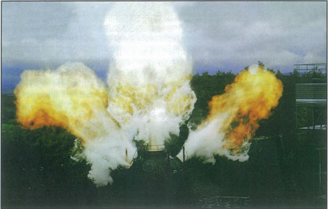
Fig. 17: Explosion venting of a 250 m 3 vessel Less rapidly developing dust explosion ( K_{St} -value = 200 bar · m · s -1 ) in a vessel with a large venting area results in a relatively low value for the reduced explosion overpressure, but causes a secondary explosion outside the vessel with not inconsiderable pressure effects (see also Fig. 18)
